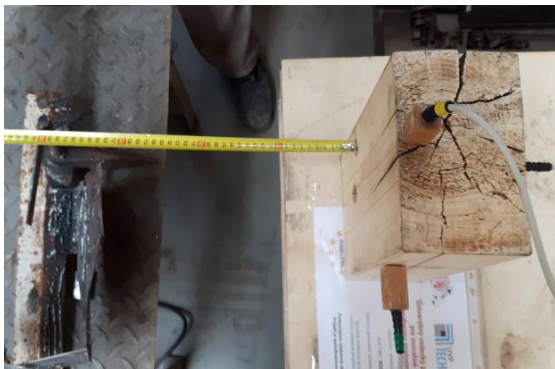
Figure 2. Measuring prism with inductive sensors
