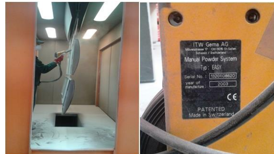
Figure 4. Powder coating chamber and powder gun label
