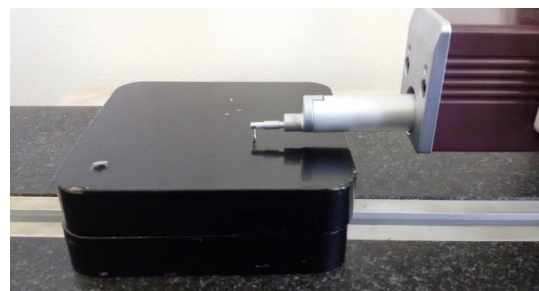
Figure 5. Measuring of surface roughness
