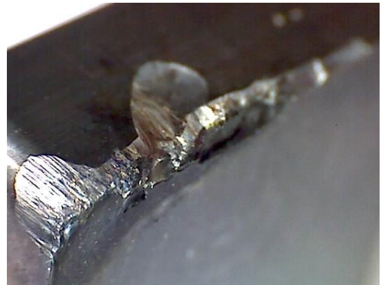
Figure 7. Wear of cutting plate
