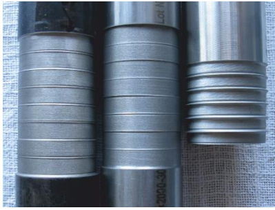
Figure 4. Turned surfaces of metals (from the left: Monel, titanium, Incoloy)
