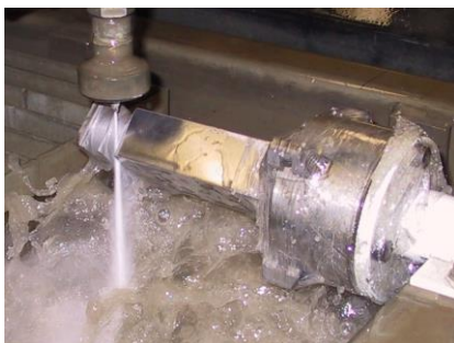
Figure 5. Turning of Inconel bar
