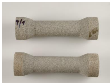
Figure 2. Testing samples turned from sandstone
