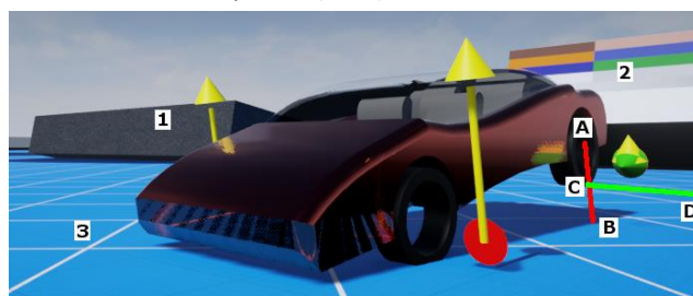
Figure 2. Contact with terrain after a jump, and line-tracing. 1 – jump ramps, 2 – rough terrain, 3 – flat terrain, A – upper end of wheel spring-dumper unit, B – terrain, C – bottom of wheel, D – line tracing in horizontal direction. AB distance is used in RK4, CD – can be used in future to improve model's abilities.
