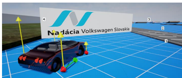
Figure 1. Virtual test facility: 1 – test road with obstacles, 2 – rough terrain, 3 – jump ramps, 4 – glass barrier and billboard
