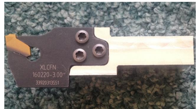
Figure 16. Prototype of new tool holder with CNC tool
