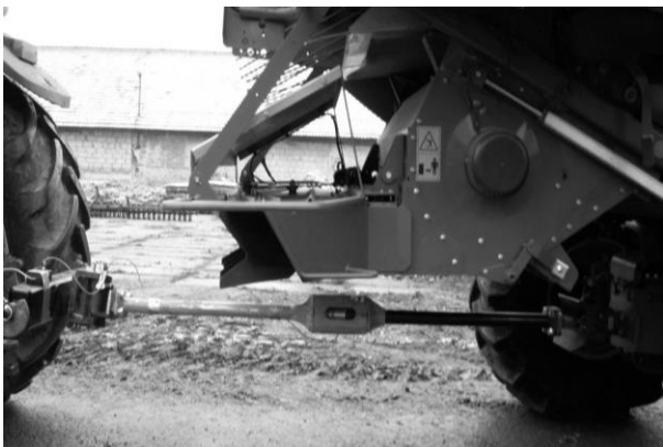
Figure 4. Measuring equipment between combine harvester and tractor
