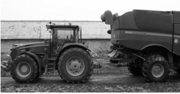
Figure 3. Measuring set. From left: pulling tractor John Deere 7930, measuring instrument, pulled combine harvester John Deere S685i without header
