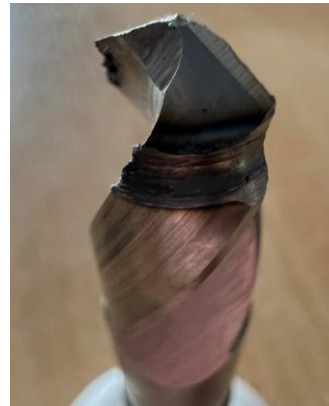
Figure 9. Wear of drill bit after drilling into C45 steel
