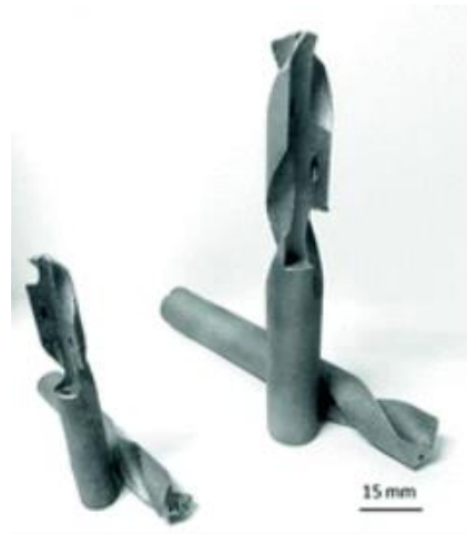
Figure 6. Printed drill bits with internal coolant channels [Zumofen 2017]
