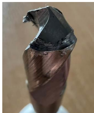
Figure 10. Wear of drill bit after drilling into Aluminium alloy
