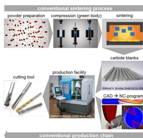
Figure 1. Conventional process of cutting tools [Schwaneckamp 2016]
