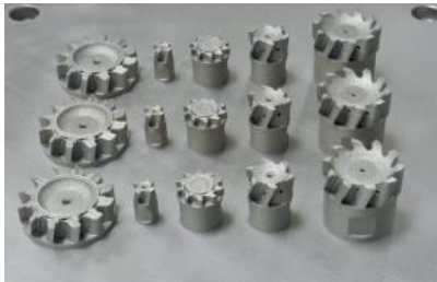
Figure 4. Printed bodies of milling tools [Klingauf 2017]
