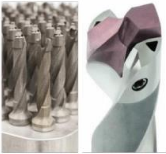
Figure 3. Indexable insert drill manufactured by SLM [Schwanekamp 2016]
