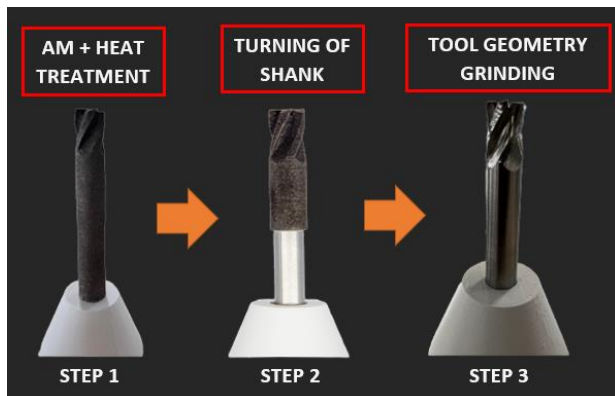
Figure 8. Preparation of tool step by step
