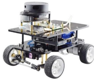
Figure 9. A mobile robot equipped with Lidar and Jetson Nano.
