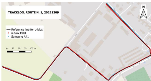
Figure 3. Visualization of point track logs from the u-blox module (red) and from the Samsung smartphone (blue) together with the reference line (black). Route number 1, drive realized on December 9, 2022. Background map: OSM ( https://www.openstreetmap.org/ ). Track logs from the other two drives on the route are comparable.
