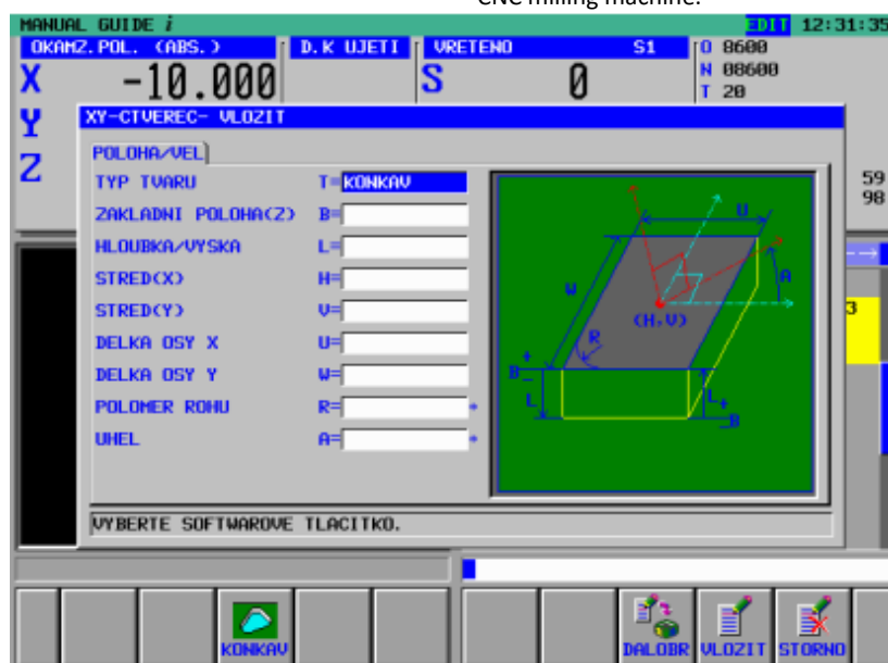
Figure 3. Working window of cutting conditions for a CNC milling machine [Michalik 2016, Sorocin 2022]
