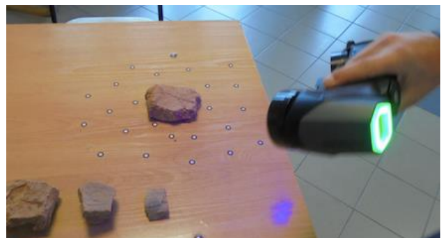
Fig. 7: The objects scanned with HandyScan3D.
