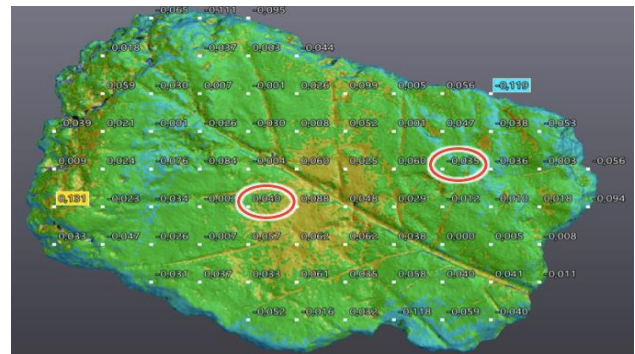
Fig. 10: The scanned object with a grid of the tested points.
