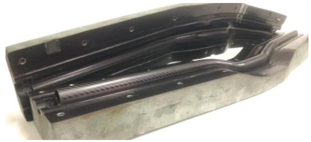
Fig. 9: The obtained CFRP handlebar and the composite mold.
