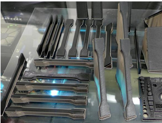
Figure 4. Specimens after print.
