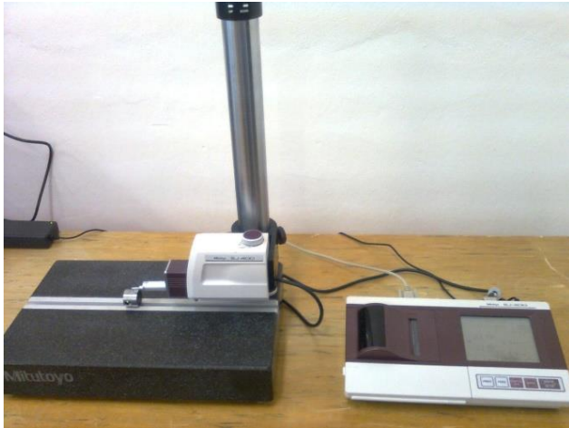
Figure 2. Profilometer MitutoyoSurfTest SJ400
