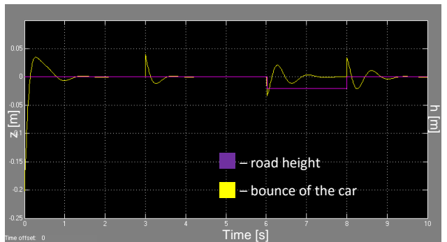
Figure 14. Graph of the waveform of the vertical reaction of the vehicle to acceleration and collision with the pothole
